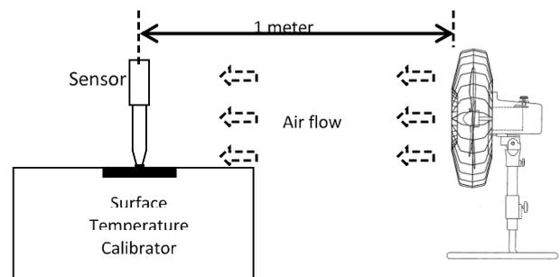
Fig 4: Sketch of the experimental setup of measuring the surrounding air velocity with forced airflow.
