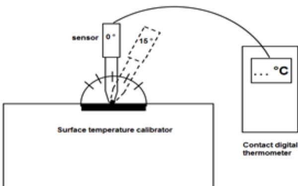
Fig 3: Sketch of experimental setup of orientation of sensor
