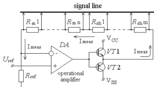
Fig. 2. Electrical schematic diagram of the current stabilizer with a circuit of Peltier modules and current shunts
