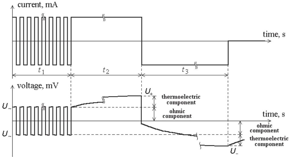
Fig. 1. Diagram of current and voltage on the Peltier module, illustrating the method of Harman measuring thermoelectric efficiency
