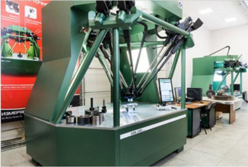
Figure 2 - measurement of geometric parameters of the Butress gauge-tube according to API 5B on the coordinate measuring machine KIM 1400 with interference sensors of LAPIK LLC»
