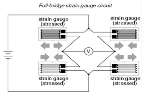
Fig. 2 – Four strain gauges in a Wheatstone bridge configuration [1].
