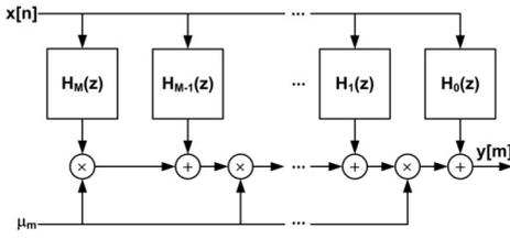
Fig. 3. The Farrow structure diagram
