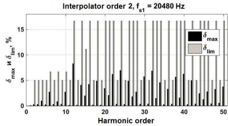
*Fig. 6. Maximum and permissible errors of the amplitude spectrum*
