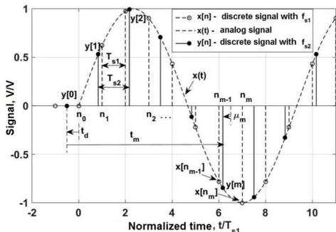
Fig. 1. Time relations between the original and the output samples of the ASRC
