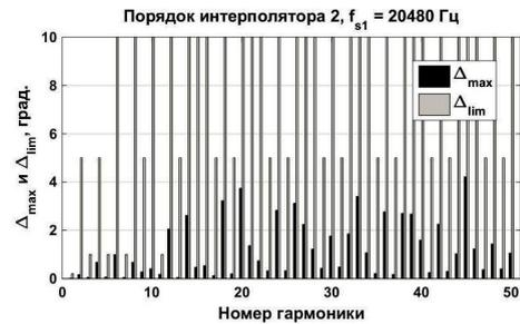
*Fig. 7. Maximum and permissible errors of the phase spectrum*
