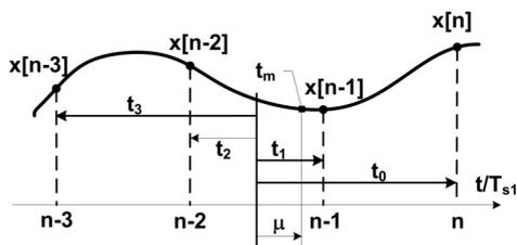
Fig. 2. The system of counting the nodes of the base points (for the variables  $\mu$  and  $n$ , the index  $m$  is omitted)
