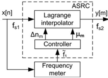
Fig. 5. ASRC structural diagram
