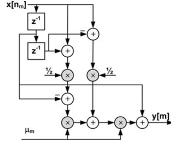
Fig. 4. Modified Farrow structure for Lagrange interpolator of the second order
