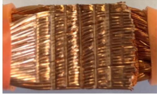
Figure 4: Illustration of visual aspect of the welding joint from anvil side
