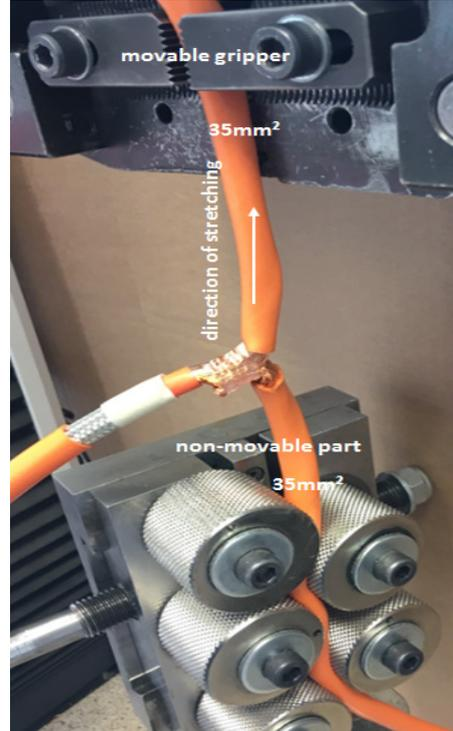
Figure 2: Illustration of Peel (share) test performing of splice with wires combination - left side: 1 time 25 mm<sup>2</sup>, right side 2 times by 35 mm<sup>2</sup>. Due to splice topology the Peel test is performed, sharing the 2 wires by 35 mm<sup>2</sup>.
