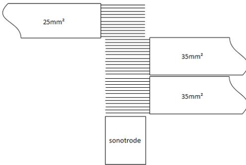
Figure 2: Illustration of sequence of wires placement (arrangements) in terms of sonotrode position.
