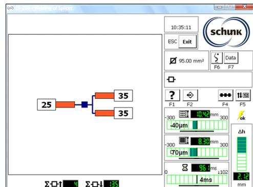
*Figure 1: Illustration of user menu with the UWW program, with the combination of wires that will be welded ultrasonically, total splice cross-section 95 mm<sup>2</sup>.*
