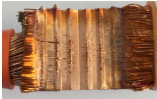
Figure 5: Illustration of visual aspect of the welding joint from sonotrode side
