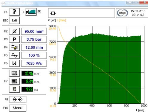
Figure 6: Illustration of Power curve
