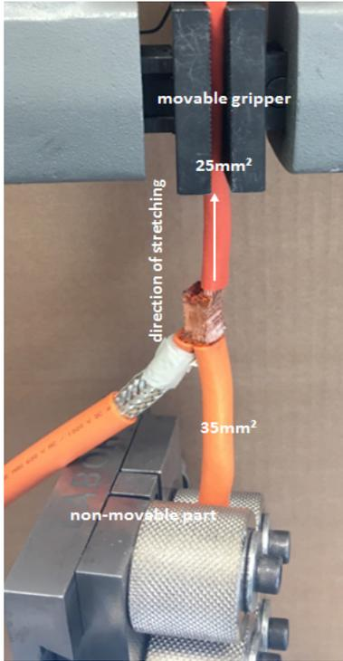
Figure 3: Illustration of Pull out test performing of splice with wires combination - left side: 1 time 25 mm<sup>2</sup>, right side 2 times by 35 mm<sup>2</sup>. Total splice cross-section 95 mm<sup>2</sup>. Due to splice topology the Pull out test is performed, sharing the 2 wires: 35 mm<sup>2</sup> and 25 mm<sup>2</sup>
