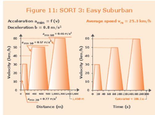
Fig. 1 Sort cycles according UITP SORT 2014, source UITP PROJECT SORT [2]
