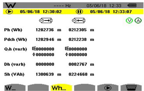
Fig. 8 Energy Record for a SORT cycle
