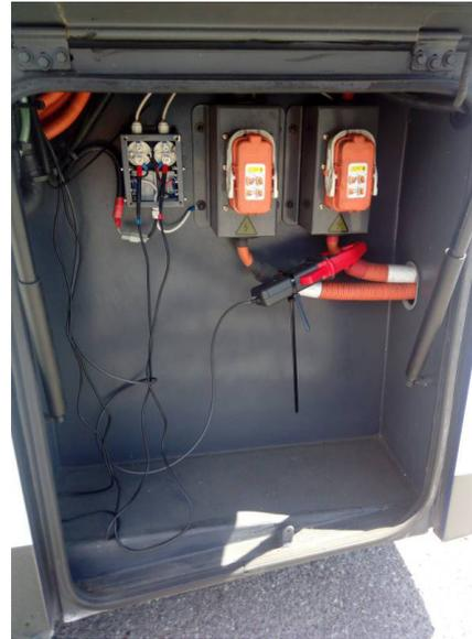
Fig. 4 connection to the RESS.
