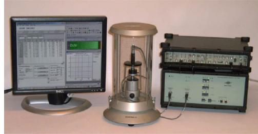
Figure 7 Recoil Calibration System for Microphones
