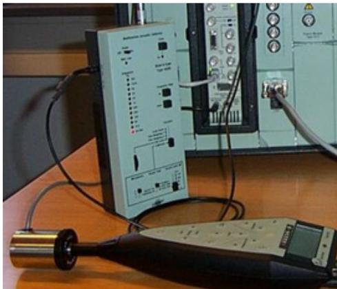
Fig. 4 Automatic acoustic calibration - sound level meter 2238
