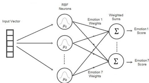
Fig. 1. Neural network for 5 features and 7 emotions accepted as the basic ones
