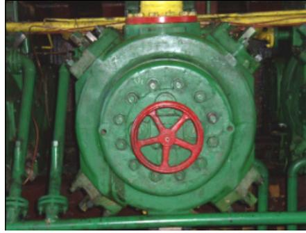
*Fig. 1. Compressor Cylinder (5 units per plant)*
