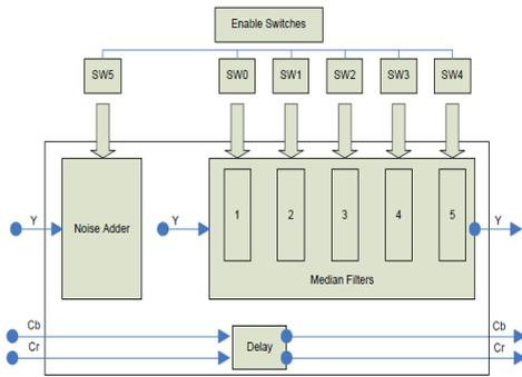
Fig.9 Noise removal system
