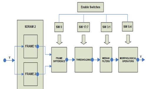
Fig.11 Motion Detector Blocks
