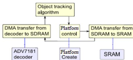
Fig. 8. Structure of the digital system
