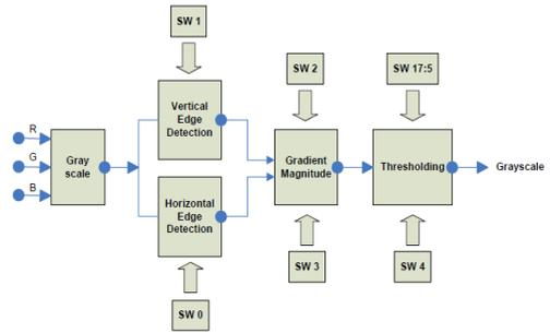
Fig. 10 Block diagram of the boundary detector:
