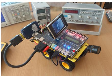
*Fig.1 The Altera De2 FPGA system*
