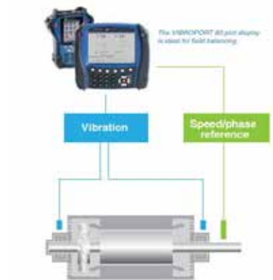
Fig. 4 – Field balancing using Vibroport 80
