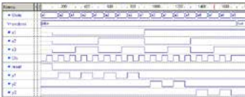
Fig. 10. Timing diagram of Moore FSM with missing transition
