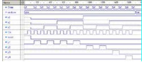
Fig. 5. Timing diagram of Moor FSM with correct conditions of transitions
