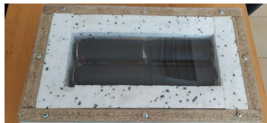
Fig.14. Final view of the assembled Panel with Plexiglas
