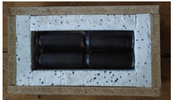
Fig.12. Panel after laying the aluminum pipes
