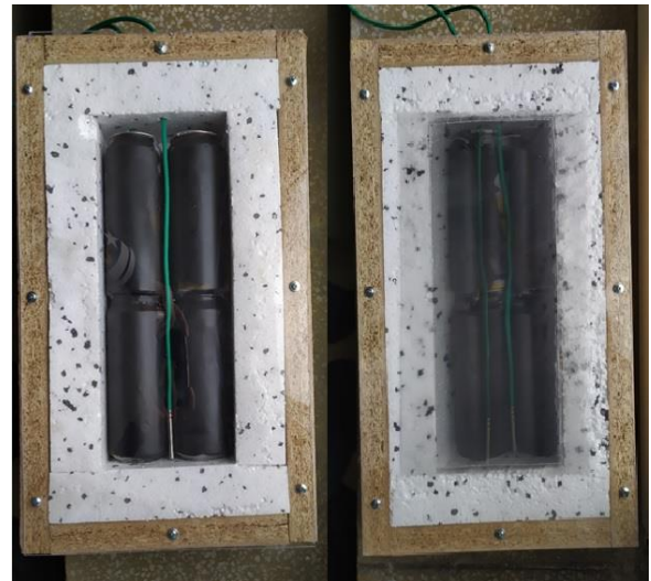
Fig.16. Front view of the finished panels (on the left panel with Plexiglas, on the right panel with Fresnel lens)
