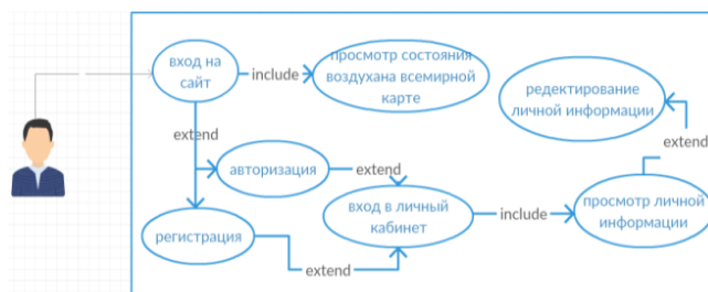
Fig.4. Usecase website diagram (Sign in, viewing air condition on the world map, editing Personal Information, authorization, registration, login into account, viewing personal information)
