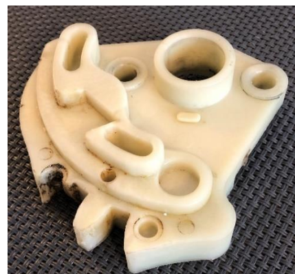
Fig. 2. A damaged part from a shift lever assembly.
