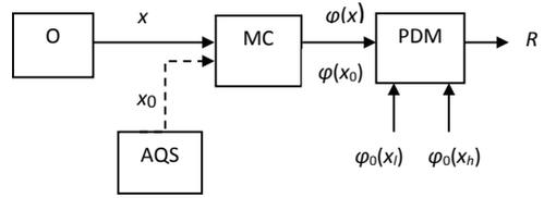
Fig. 1. Method for increasing the reliability of measurement inspection: O – controlled object; AQS – auxiliary quantity  $x_0$  source; MC – measuring channel; PDM – processing and decision making module, R – result of inspection
