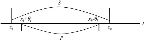
Fig. 2. Location of the intervals of parameter  $x$  for the objects which met efficiency standards  $S$  (tolerance interval) and found as fit  $F$  (acceptance interval)
