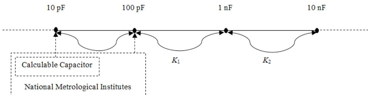
*Fig. 1. The transmission of the unit size of capacitance over the value range*
