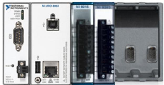
Figure 5 Rack NI cRIO-9063 with NI9215 and NI9263 modules
