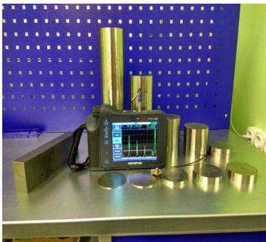
Figure 4 – Thickness gauges
