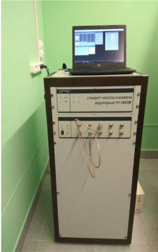
Figure 6 – Hydrogen time and frequency standard
