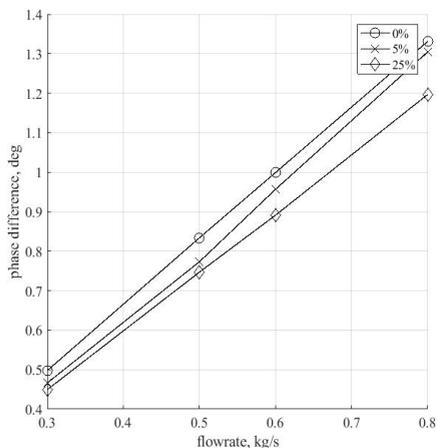
*Fig. 2 – The GVF impact to transducer CC*
