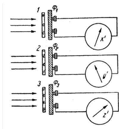
Figure 1 - Schematic diagram of the objective colorimeter
