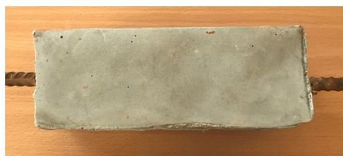
Fig.1. Appearance of the reinforced concrete sample before the tests
