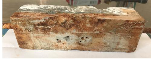
Fig 4. Sample after electrocorrosion
