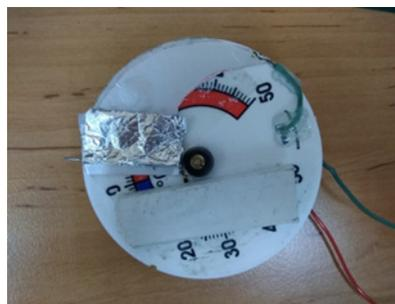
*Fig.4. Capacitive floating electrode a pin and rectangular shaped aluminium foil.*
