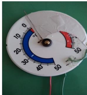
*Fig.3. Capacitive transducer with floating electrode one pin.*
