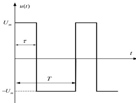
Fig.2. Timing diagram of periodic bipolar squarewave signal
