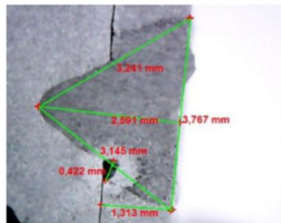
Fig.2. Shape of the weld seam.
