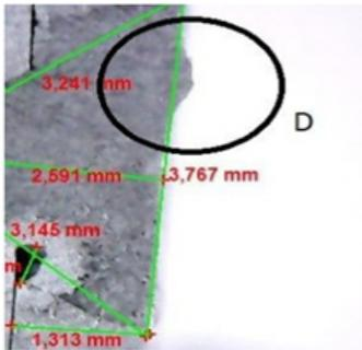
Fig.3. A protruding section of the weld seam.
