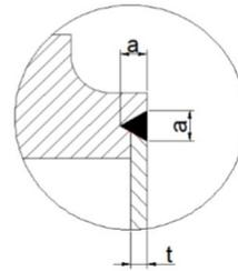
Fig. 1. Geometric parameters of the weld seam.
