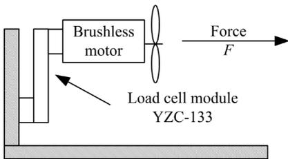
Fig. 2. The schematic diagram of the thrust MC construction
