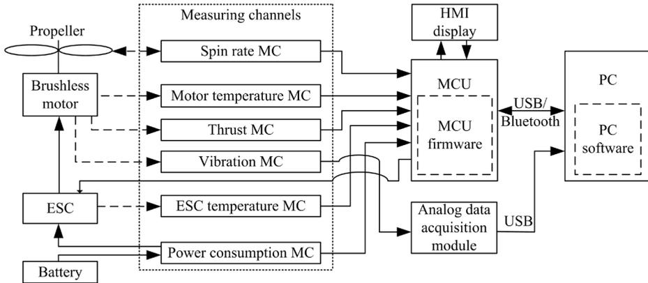
Fig. 1. The structural schematic of the testing workbench
