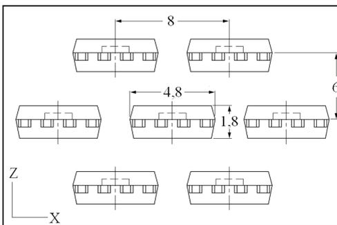
Fig.3. 7-element hexagonal array.
