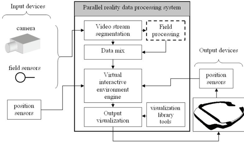
Fig.1. Augmented reality system block scheme.
