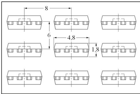
Fig.2. 3x3-element square array.
