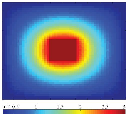
Fig.4. Calculated  $B_y$  distribution.
